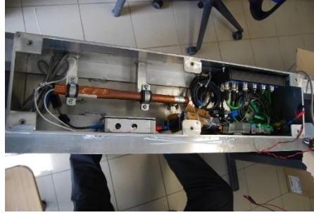
FIGURE 6. Picture of the heat flux micro-sensor, converter and acquisition integrated in the scanning bar
