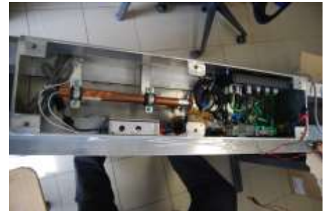
Acquisition system installed at the back of the moving bar
