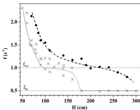
**FIGURE 7:** Bubble and/or slug frequency,  $f$  ( $s^{-1}$ ) versus level in the bed,  $x$ : ambient temperature,  $\bullet$ : at 475 °C.
