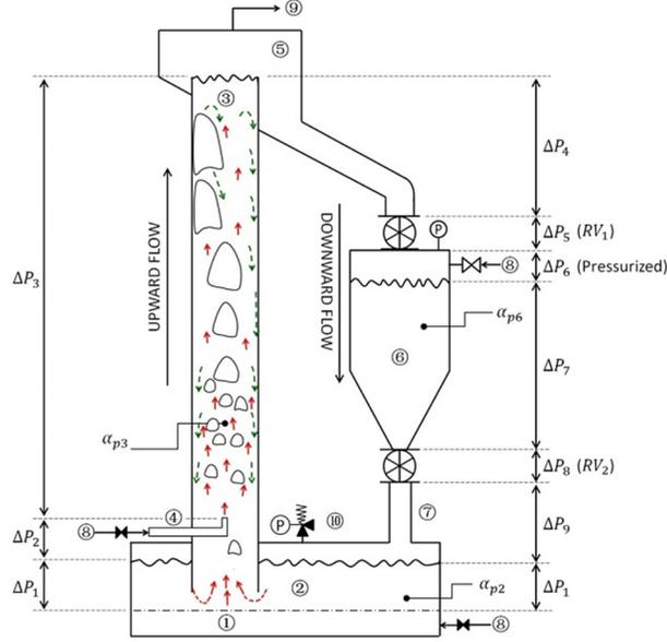
**FIGURE 4:** Particle movement and pressure balance in the UBFB<sup>7</sup>, with bubble and  $G_s$ -driven particle upflow; gross particle downflow near the wall; ① windbox; ② fluidized bed dispenser with ⑩ pressure relief valve; ③ up-flow bubbling fluidized bed; ④ secondary air injector; ⑤ disengagement chamber; ⑥ pressurized hopper; ⑦ downcomer; ⑧ compressed air; ⑨ to fines filtration. RV: rotary valve
