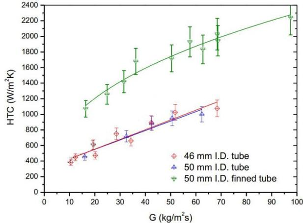
FIGURE 3: Experimental heat transfer coefficient versus solids circulation flux  $G$  for different tube geometries <sup>6</sup>
