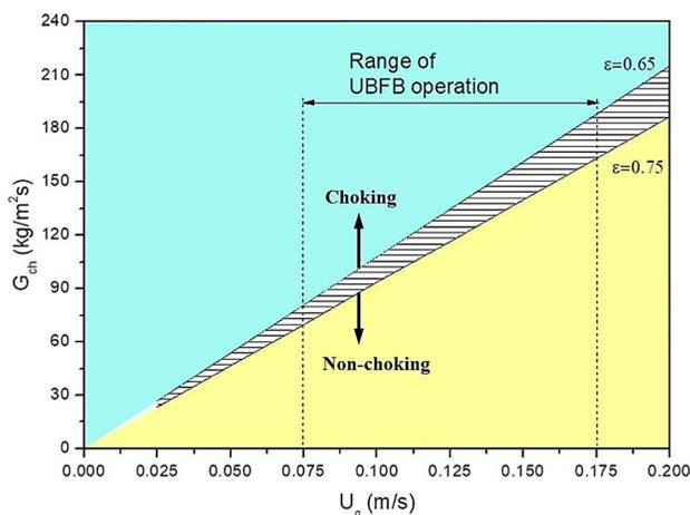
**FIGURE 8:** Predicted choking limit at different superficial gas velocities and bed voidages between 0.65 and 0.75
