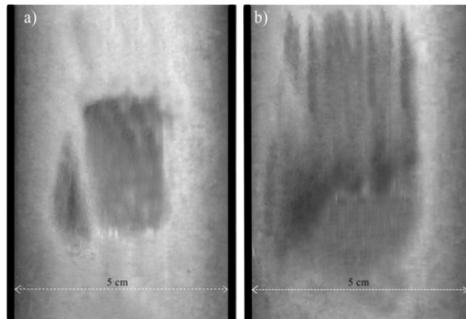
**FIGURE 6:** Wall slugs at the level of 90 cm in the bed: a)  $U-U_{mb} = 8.9$  cm/s; b)  $U-U_{mb} = 11.4$  cm/s
