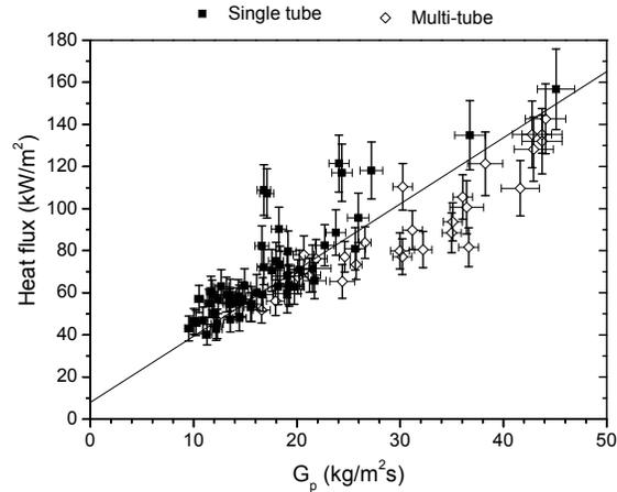
**FIGURE 1:** Heat flux vs. mass flux in single and multi-tube experiments (Credit: PROMES-CNRS)
