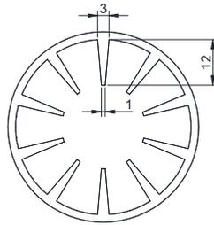
**FIGURE 2:** Top view of the 50.09 mm O.D. finned tube (dimensions in mm)
